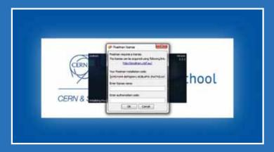
To fix this, cancel any open Pixelman windows and connect the detector to the laptop via the USB cable. Pixelman will now open as the license for use is associated to the detector itself. This means that any data analysis done using Pixelman will require the presence of a detector.
