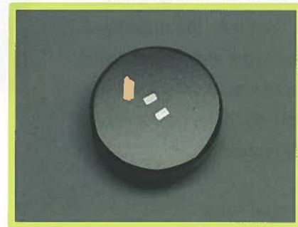
Fig. 3 Example of X-ray Analysis Specimen Mechanically Polished after Resin Embedding
