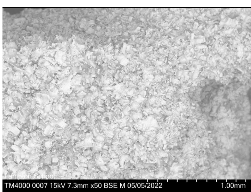
Figure 3 Calcium oxalate crystals pre treatment, x50 Magnification
