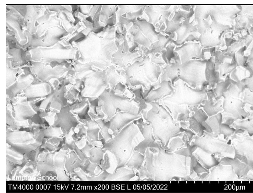
Figure 4 Calcium oxalate crystals pre treatment, x200 Magnification
