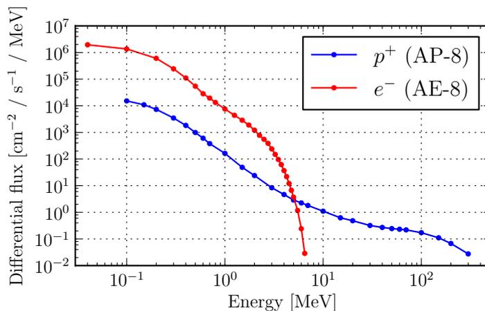
**Figure 2.** Differential flux spectra for trapped protons and electrons in TechDemoSat's initial orbit (see table 1), as estimated by SPENVIS [6] using the AP-8 [7] and AE-8 [8] models.
