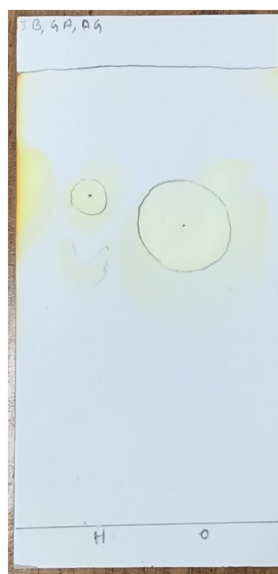
- thin layer chromatography of 1-hexylimidazolium bromide + 1-decylimidazolium bromide.
