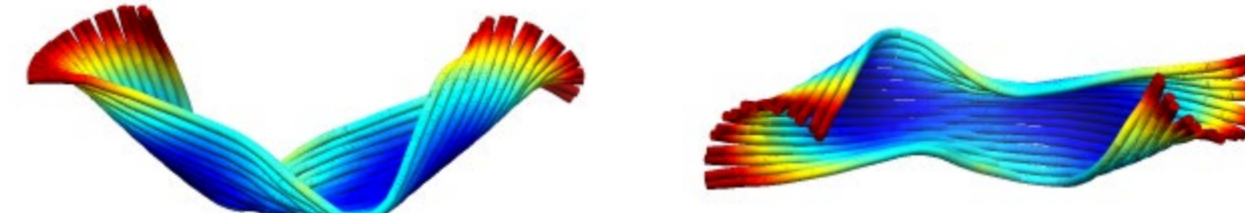
Mixing Insertions and Deletions As shown by the unusual shape of the above design, insertions and deletions can be used to create some unusual shapes. This particular design shows a similar structure to a flat rectangle which has had extra material added to its middle, causing it to bulge outwards, and fold up at the edges, which is due to the use of insertions solely in the centre of the design.
