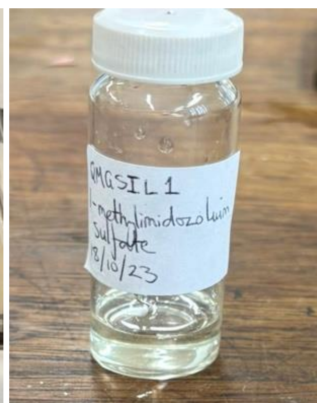
A vial of 1-methylimidazolium hydrogensulfate
