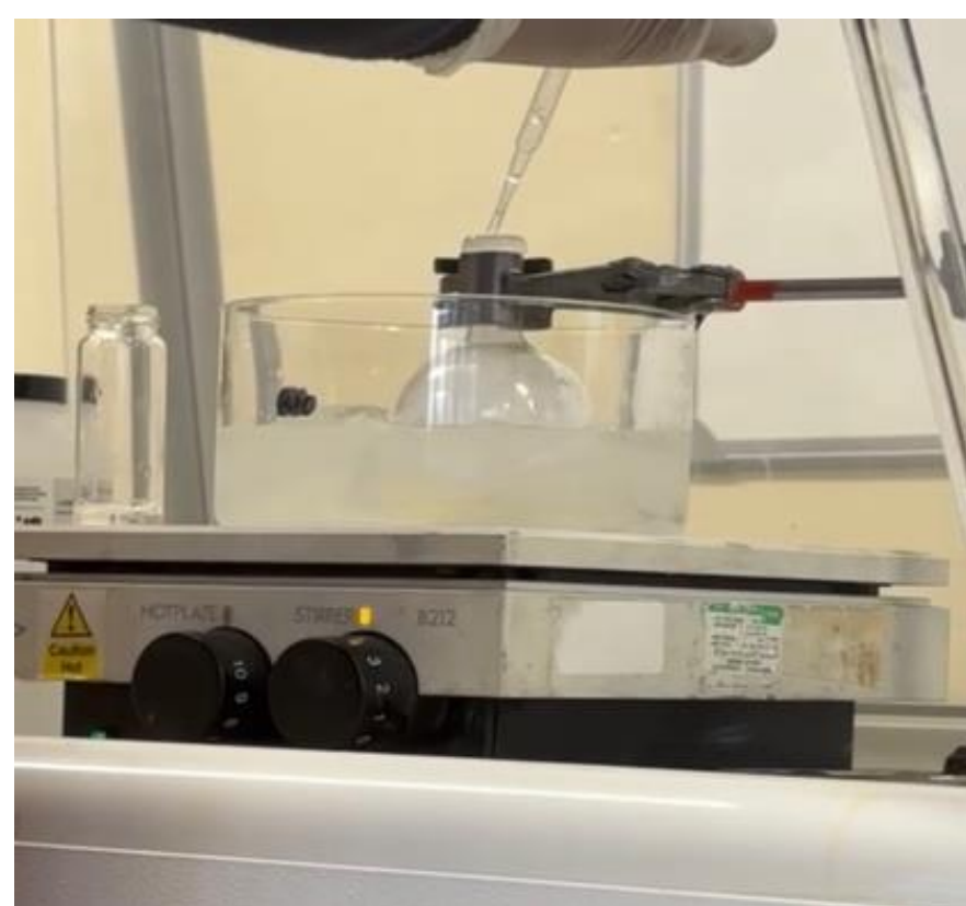
Addition of 1-methylimidazole to conc. sulfuric acid
